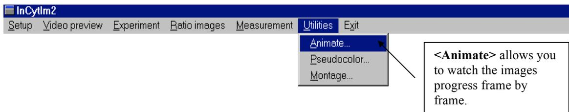
Animate is a good way to see how the changes progressed during the experiment. The animate function will replay the experiment for you frame by frame, or you can manually choose the frames you wish to view. This allows you to compare the different images that were captured during the experiment.
