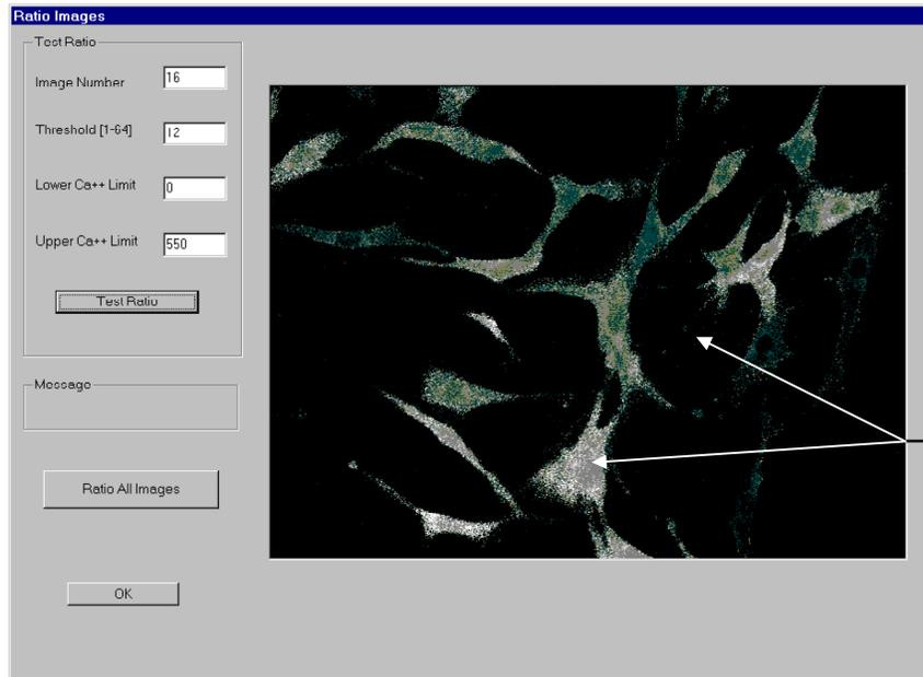
Here a threshold of 12 produces a nice dark background and clear, complete cell images. This is a good image.
