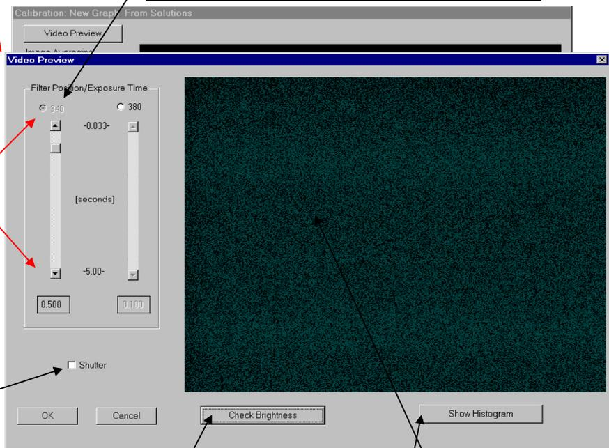
This allows you to check if any part of the image is too bright (saturated) or too dark. A saturated pixel is **RED**; a black pixel is **GREEN**. When <Check Brightness> is on, this button will read <Reset to Gray>.
