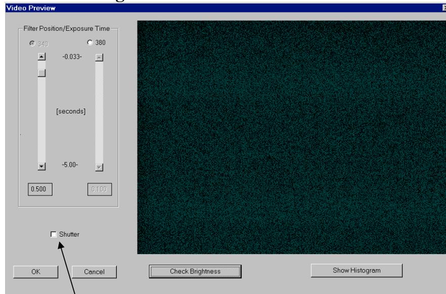
When you click on the <Shutter> radio button, the Filter Wheel is directed to find the shutter position closest to the numerator wavelength.
