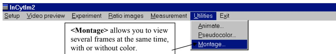
A montage is a good way to display your results. It allows you to display up to four of the images you captured from the experiment. This can help you to demonstrate the changes that occurred during the experiment or present your data in an easy to understand format. These images can be from the ratio, 340, or 380 pictures, or they can be from a variety of those 3. You can have some of the images in color and some in black and white, and you can add text to the montage.
